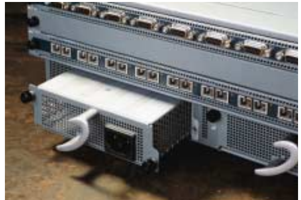
FIGURE 4 Model 3001 removable power supplies in Capellix 3000HA
